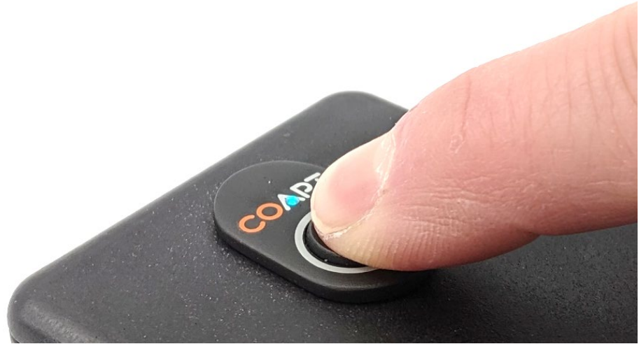
Figure 12: Pressing the COMPLETE CALIBRATE Button located on the top of Evaluation Kit main unit
