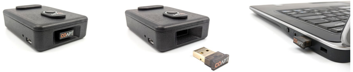
Figure 10: Preparing for Bluetooth communication by removing the COMPLETE COMMUNICATOR USB Dongle from its Evaluation Kit holder (Left-to-Center) and plugging it into a personal computer USB port (Right)
