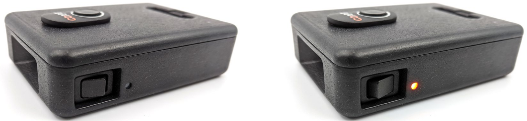
Figure 8: Evaluation Kit powered off (Left) and powered on showing the illuminated orange Power ON LED (Right)
