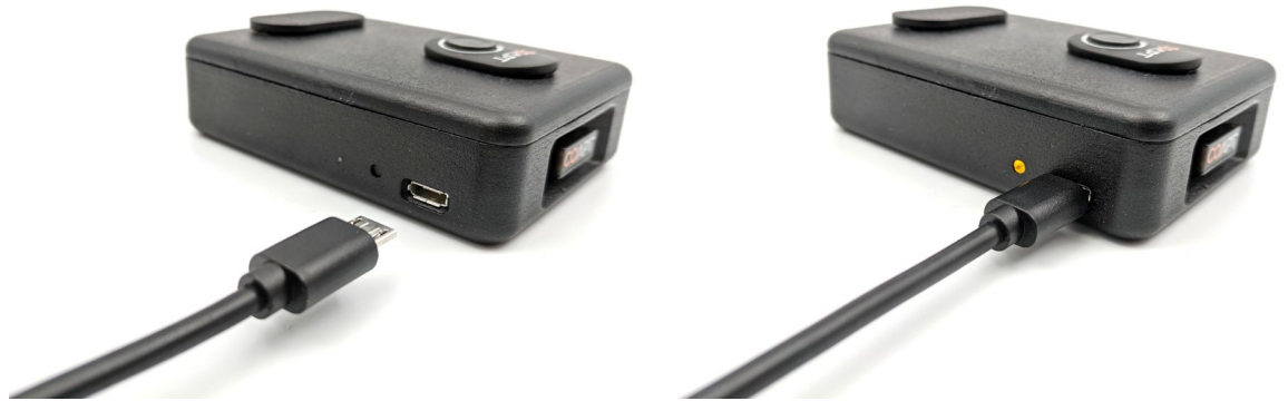
Figure 7: Evaluation Kit and micro-USB cable disconnected (Left) and connected/charging (Right)
