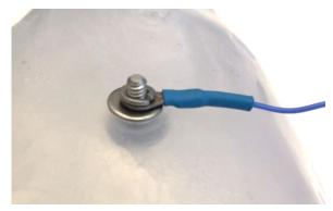
Next, a split "lock" washer is added on top of the conductor cable.
