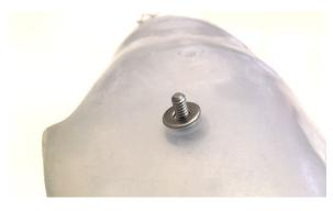
Next, the flat washer is placed on the threaded side of the dome electrode.
