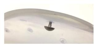
Place the Dome Electrode through the hole in a prosthesis' socket wall or enclosure of compatible device. Place it so the dome will make contact with the skin of the user, and the thread is on the other side of the socket or enclosure. The socket/enclosure also provides a way to keep the other hardware components of the electrode and connected device from contacting the user.
