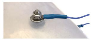
The 4-40 nut is fastened onto the threaded side of the Dome Electrode, securing all components and conductor cable to the compatible device.
